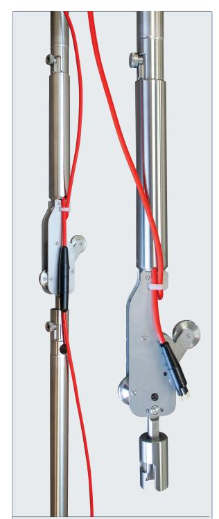
A close-up shows the signal cable which connects each sensor along the entire chain of inclinometer sensors forming a "digital bus"
