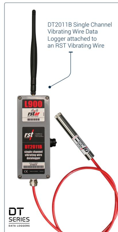
DT2011B Single Channel Vibrating Wire Data Logger attached to an RST Vibrating Wire
